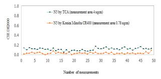
Figure 2. CIEDE2000 colour difference between measurements obtained from the TCA and Konica Minolta CR400 on Munsell grey N5 (non-homogeneous surface)
