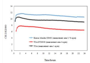
Figure 1. CIEDE2000 colour difference between measurements (1<sup>st</sup>-2<sup>nd</sup>, 1<sup>st</sup>-3<sup>rd</sup>,..., 1<sup>st</sup>-67<sup>th</sup>) over time obtained from the TCA with measuring areas of 1 and 4 sqcm and Konica Minolta CR400 with measuring area of 0.78 sqcm on fresh cut GS green apple slice
